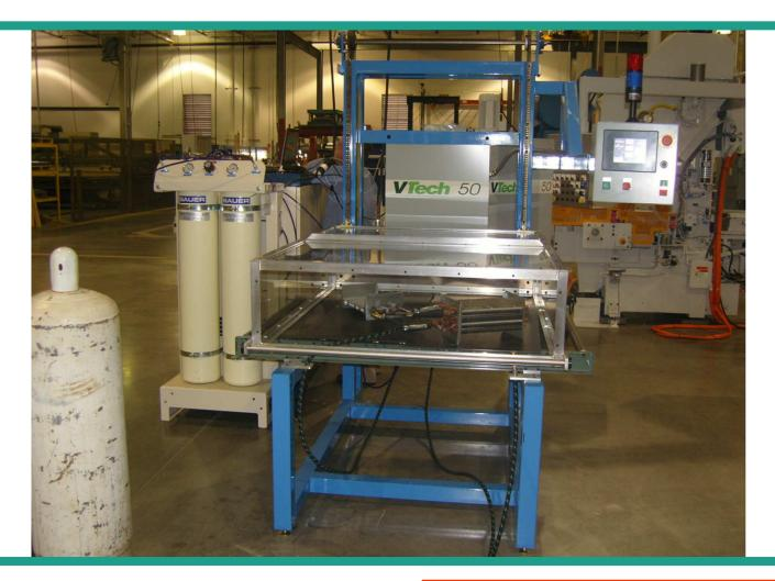
The **VTech 50 PDLT System** is designed for testing coils and other components, or sealed refrigeration systems, in a production environment. The system performs an automatic pressure decay leak test (Go-No Go) according to a pre-set cycle stored in the PLC memory. An optional capillary flow test can also be included.
